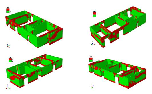
Figure 6. Cracking zone (in red) of the URM walls.
