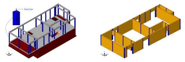
Figure 7. Seismic reinforcement solution.
