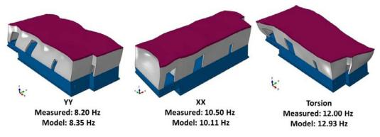
Figure 4. Calibration of the finite element model with ambient vibrations results.
