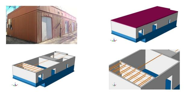
Figure 2. Geometry of the numerical model.
