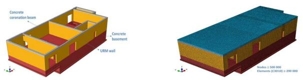
Figure 3. FE meshing of the numerical model.
