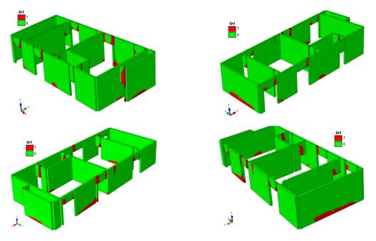
Figure 8. Cracking zone (in red) of the masonry wall after reinforcement.
